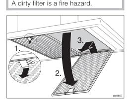
■ To remove the grease filters pull the locking clips, **1**, forward. Lower the filter 45°, **2**, unhook it at the rear, **3**, and take it out. Support the grease filter so that it does not fall onto the cooktop.
